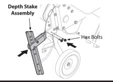
To adjust wheel height remove cotter pin from clevis pin, clevis pin from wheel yoke and slide depth stake in the yoke to the desired height. Reinstall hardware.
