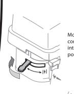
Move the choke control into the Choke position.
