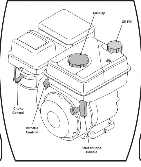
Move throttle control into the Fast **#** position.
