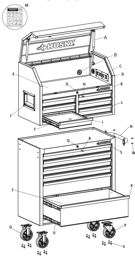
Chest Part Description Quantity **Gas Strut** Α 2 В **Rubber Grommet** 3 Outlet С 1 D **Outlet Panel Cover** 1 Ε **Drawer Liner** 7 F **Drawer Slide** 12 G Lock 1 Н 2 Key **Removable Work Table** Т 1 Side Handle 2 J Κ Badge 1 L **Drawer Handle Cap** 12 Magnetic Drawer Icon Μ 1
