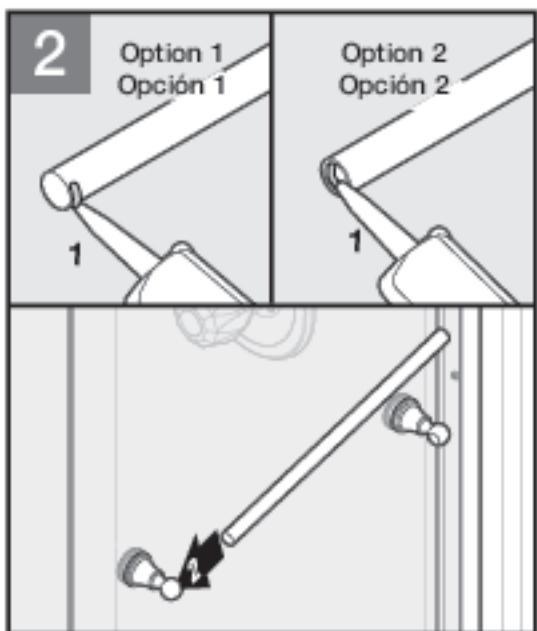
**Option 1:** For handles that insert **INSIDE** the post ends, apply a thin bead of silicone sealant onto the **OUTSIDE** bottom 1/4-inch of one end of the handle bar before inserting into the handle post. Next, install the second handle post and repeat the sealant steps. Wipe away excess sealant immediately. See sealant manufacturer's instructions for cure time, cleaning, safety and handling instructions.
