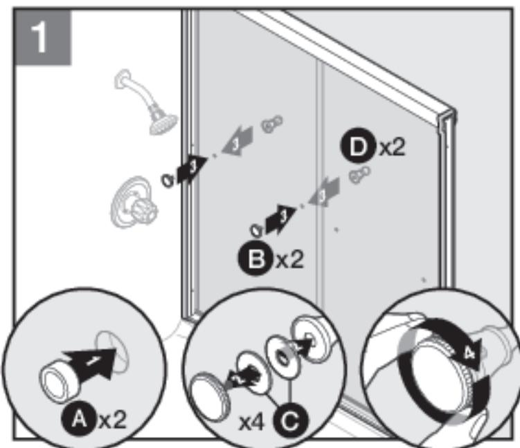
Install bushings (A) into pre-drilled holes in outer shower door. Insert a rubber gasket (C) to handle post (B) and escutcheon (D). Install escutcheons into bushings in pre-drilled holes in shower door. Secure escutcheons manually. **IMPORTANT: DO NOT** overtighten. Using tools to tighten is not recommended.
