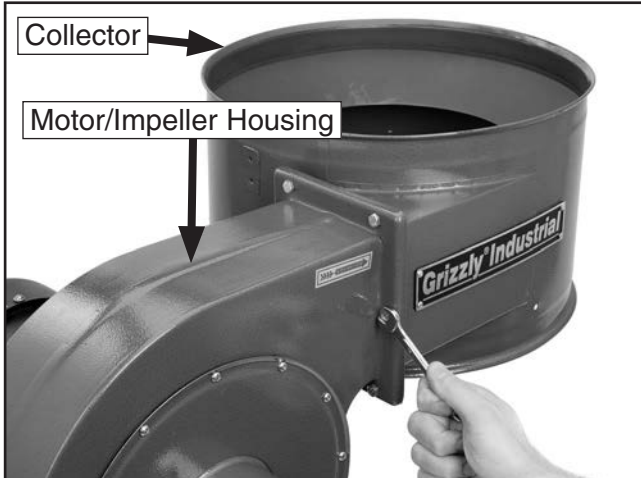
Figure 8. Installing collector onto motor/impeller housing.
