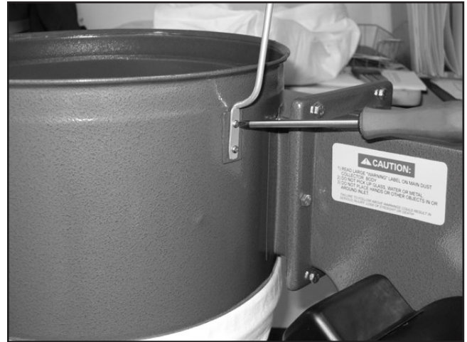
Figure 10. Installing upper bag support.
