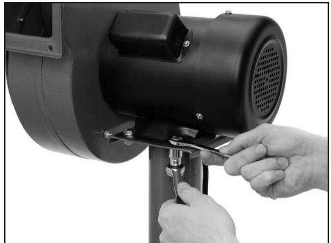
Figure 7. Installing motor/impeller housing on collector support.
