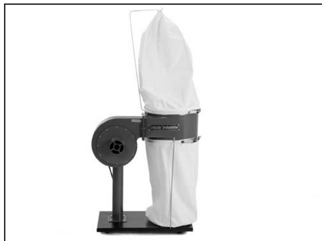
Figure 14. Filtration and collection bags installed.
