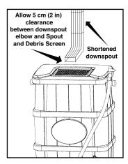
The Before positioning the barrel, you will need to shorten the current downspout to allow water to exit into the barrel. Remove elbow from bottom of downspout, measure and cut the downspout so that it will be 5 cm (2 in) above the barrel screen once elbow is reinstalled.
