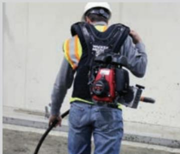
These gasoline vibrators feature high impact, high frequency concrete vibration. Portable vibrators are ideally suited for light to medium duty concrete work and hard to reach concrete applications. Offering over 10,000 vibrations per minute, these vibrators are portable and productive... a winning combination for any jobsite.
