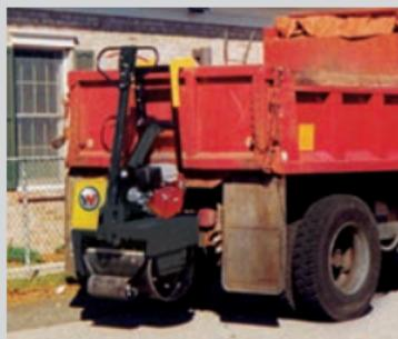
Lightweight and highly maneuverable roller has infinitely variable hydrostatic drive with high curb clearance and close side clearance.
