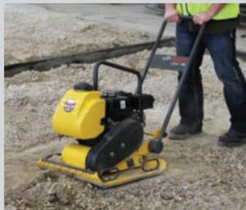
These plates are optimally suited for a variety of compaction applications thanks to their high speed and simple maneuverability. The asphalt plate models feature a large capacity water tank and wide filler opening. Plates feature a baseplate width of 19.5 inches.
