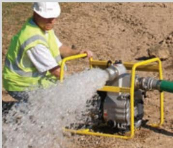
Centrifugal pumps designed to keep your job site dry. With its radial flow design and built-in contractor friendly features, this line of trash pumps have redefined the quality and durability standards of self-priming centrifugal trash pumps. These 3-inch trash pumps can handle solids up to 1.5 inches.
