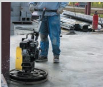
Specifically designed for up to the edge finishing, this compact trowel eliminates hand work along walls. This machine improves productivity and quality while providing more ergonomics for the operator. Offering better floating and finishing capabilities along wall lines and obstacles, the CT 24-4A edging trowel delivers an unmatched solution to the concrete job site.
