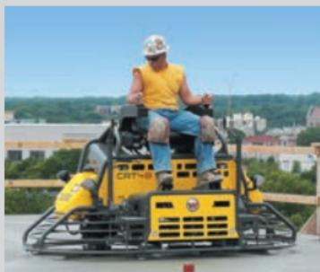
This innovative trowel combines hydraulics and electronics to offer a true power steer system that offers the results of a hydrostatic unit matched with the responsiveness of a mechanical steer unit. Ideal for large pours and on elevated deck pours where lighter weight machines are preferred. Patented dual mode steering program to switch from settings for large open areas and for use in tight clearance areas around slab obstructions.
