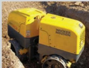
Articulated trench roller features a dual joystick control and smart infrared remote control system for added safety. The extendable drums allow the machine's width to be converted from 32" to 22" wide.
