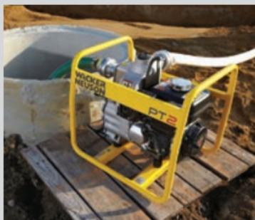
These centrifugal trash pumps have proven themselves on job sites around the world. Pumps feature hardened ductile iron impeller and volute with patented pump cover, volute and volute insert providing a rugged, easy to maintain pump that will stay on the job longer. Units can handle solids up to 1.0 inch.
