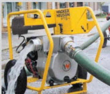
Self-priming, high performance pump capable of handling solids up to 2 inches, ideal for job sites requiring fast dependable dewatering on command. Featuring electric start and a thread-on mixed flow impeller design.
