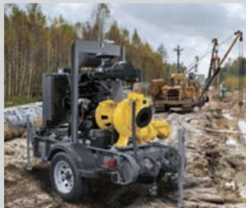
The Wacker Neuson automatic self-priming centrifugal trash pump is the perfect pump for contractors, pump rental companies, mining operators, general industrial and municipal use. High-grade cast ductile iron pump housing, wear plate, and impeller construction makes this unit jobsite tough.
