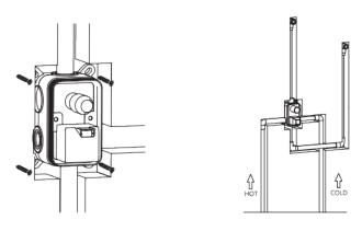
3.Stick the tiles and cut off the edge of the installed box, Remove the protective cover and install the panel
