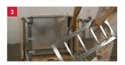
**Step 3:** Place Support Rack. Make sure to place the tank holder facing the right side of the unit so once propane tank is placed it lies directly underneath the gas valve hose.
