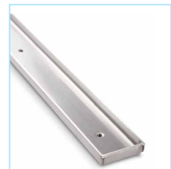
13 Exclusive tileable drain cover for Fundo Riolito: can be tiled with epoxy glue/adhesive or wedi Joint Sealant- used with 1/4 inch and 1/2 in. tile/stone (reverse cover). Drain cover can be adjusted from +3/16 in. to +1 in. from the Riolito base surface.
