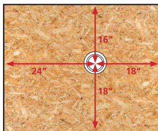
Offset drain location in 34 x 42 in. shower area
