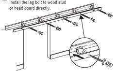
Insert door stoppers into rail, install door stoppers between A-B and C-D. Door stopper is used to prevent the hangers coming out of the rail.
