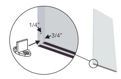
Install the hangers onto the door according to the measurement in the pictures below. Maximum door thickness is 1 3/4", please add some bolt washers or cut the long door bolts to a suitable length to fit the door.
