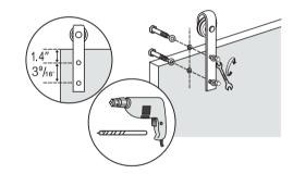
The rubber ends are used to protect the door from touching the rail when sliding the door. You need to drill holes on the door top side, please drill the holes 1/2 away from the edge of the door. Then install the rubber ends on the door.
