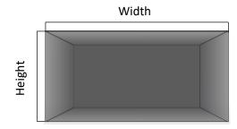
**Step 1** - Measure the opening over which the register needs to be installed. For rectangular openings measure the width and height of the opening in inches. For square openings, measure one of the sides in inches.
