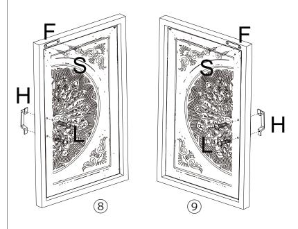
Attach magnet sheet (F) to door (8.9) using screw (S) Attach handle (H)to door (8.9) using screw (L)
