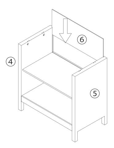
Slide back panel (6) to the groove as diagram
