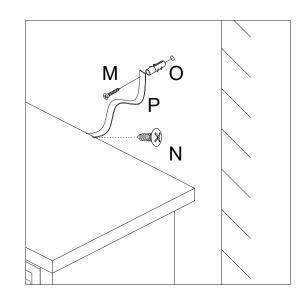
Drill 2 holes on the wall, Insert nut (O) into the wall.
