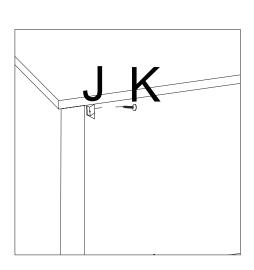
Lock the back panel (6) to frame using panel hook(J) and screw (K)
