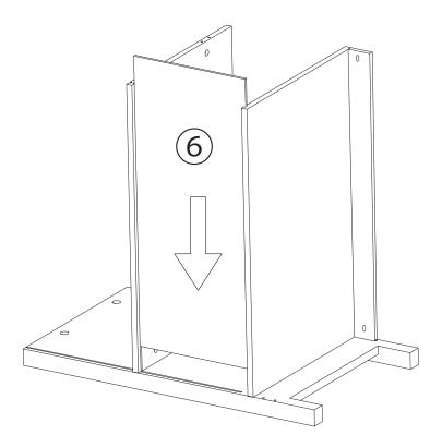
Slide back panel (6) to the groove as diagram
