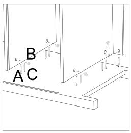
Attach cam bolt (A) and wooden dowel (C) to panel (5) Attach panel (1.3) to panel (5), insert and secure with cam lock (B) A x5 B **a** x5
