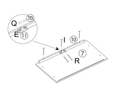
Attach magnet (E) to panel (11) using screw (Q) Attach panel (11) to panel (10) using screw(R) Attach panel (10) to panel (7) using secure (I)
