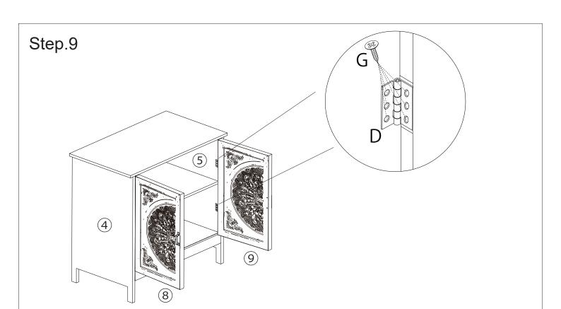
Attach door (8.9) to finish unit by Step 8 by hinge (8), lock it by screw (G)
