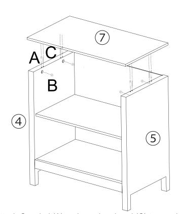
Attach Cam bolt(A) and wooden dowel (C) to panel (7)
