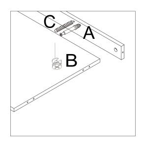
Attach cam bolt (A) and wooden dowel(C) to panel (2)
