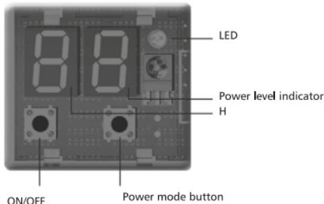
The LED panel on the body of the UK heater allows you to turn the unit ON or OFF and set the power level. No programmed or timer operations can be initiated from the LED panel.
