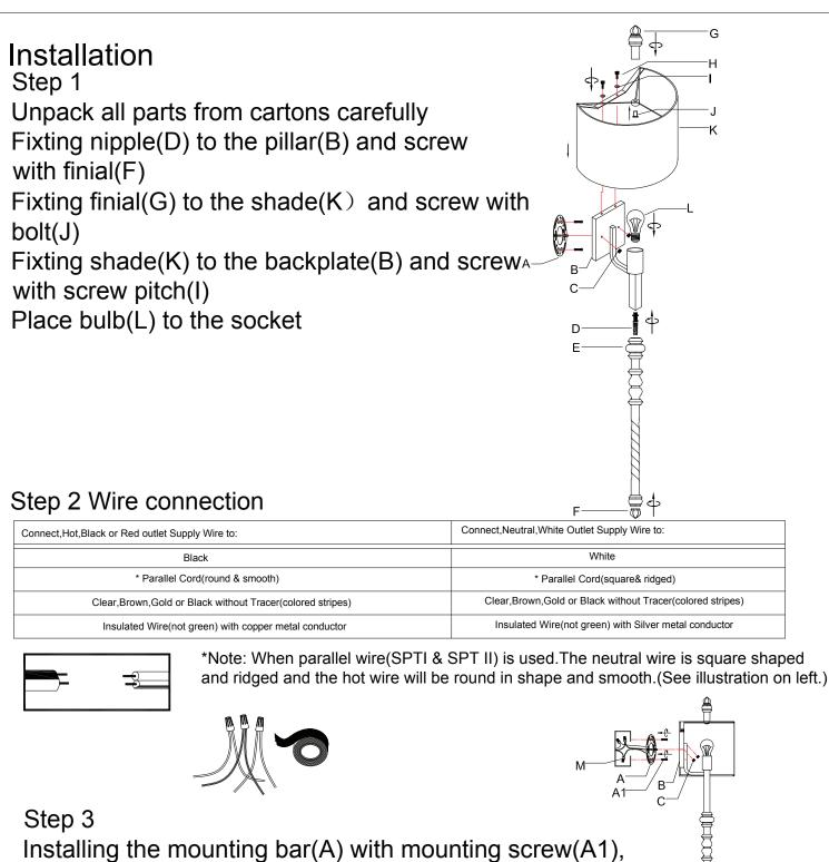
and secure Backplate (B) with Backplate screw(C)
