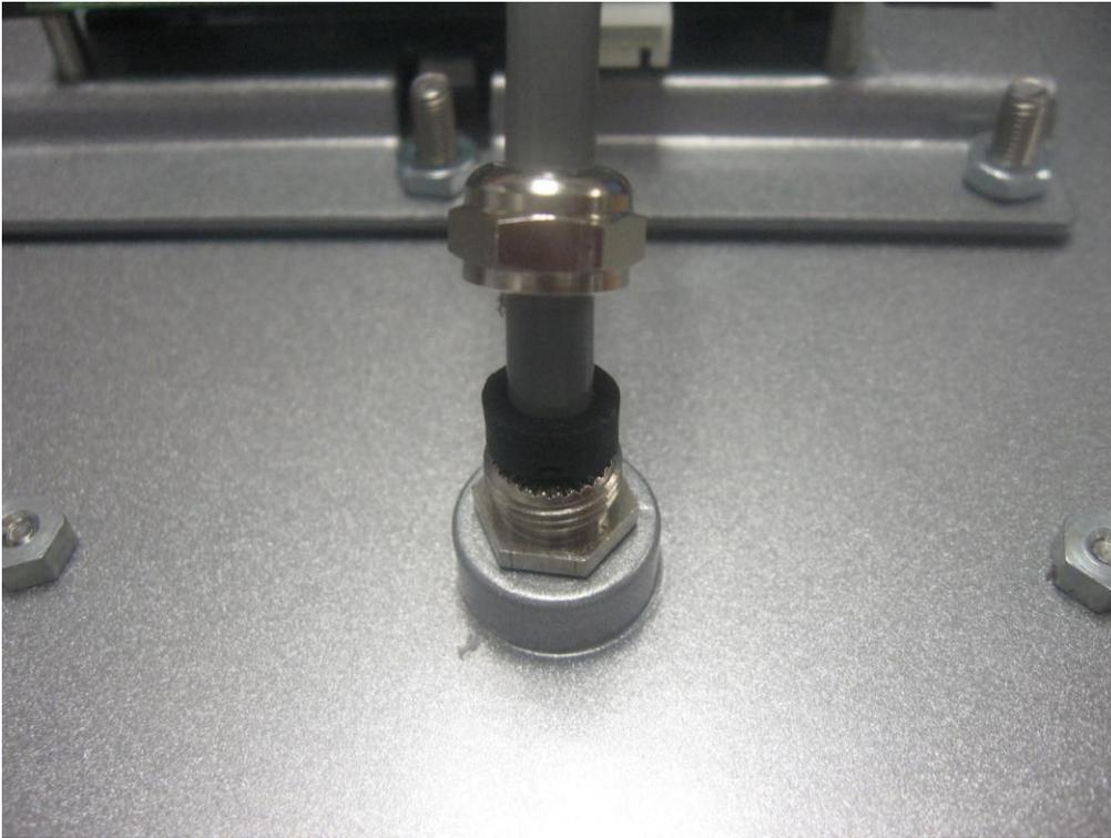
Figure 37: RFID gland assembly
