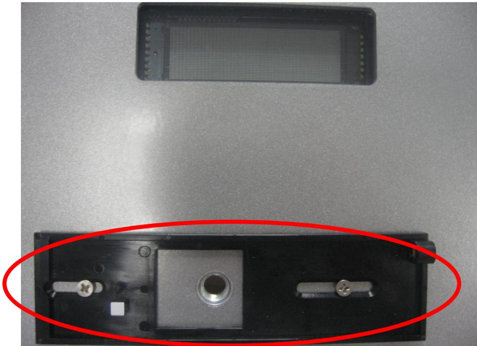
Figure 33: RFID mounting plate, outside view
