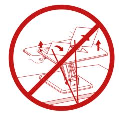
MAKE SURE devices have cables long enough for the full-range (11.8 in/29.9 cm) of height-adjustment.
