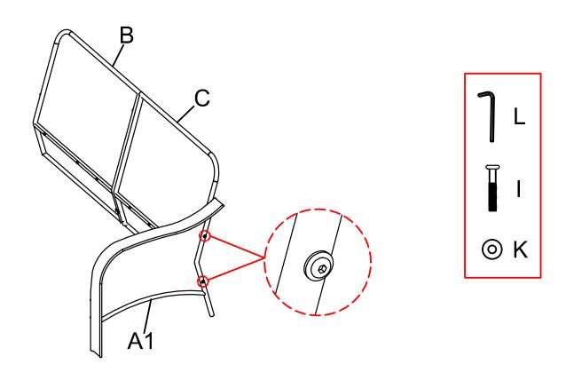
**Step 4**: Attach right arm A2 to back panel B with 2pcs bolts I and 2pcs washers K,using Allen wrench L .Note: Don't fully tighten the bolts.
