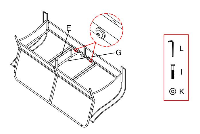
**Step 9**: Attach seat to back panel with 6pcs bolts I and 6pcs washers K ,using Allen wrench L. Note: Don't fully tighten the bolts.
