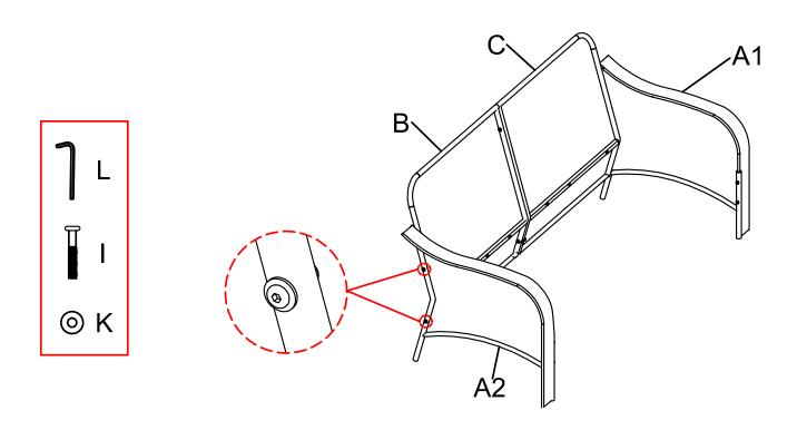
**Step 5**: Attach front panel D&F to arms A1&A2 with 4pcs bolts I and 4pcs washers K,using Allen wrench L. Note:Don't fully tighten the bolts.
