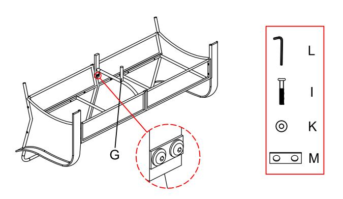
**Step 7**:Attach Middle foot G to Middle seat E with 2pcs bolts H and 2pcs washers K,using Allen wrench L .Note: Don't fully tighten the bolts.
