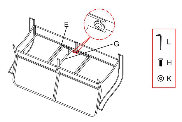
**Step 8**: Attach middle seat E to front panel with 2pcs bolts I and 2pcs washers K ,using Allen wrench L. Note: Don't fully tighten the bolts.
