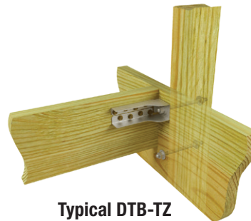
Typical DTB-TZ deck to ledger installation
