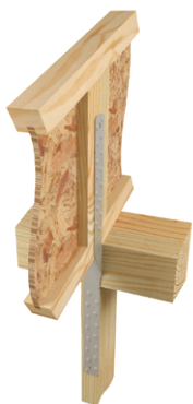
Typical MTW20 I-joist rafter installation
