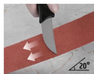
1. Instead of leading with the cutting edge, you will drag the cutting edge back across the leather strop.
