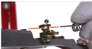
8. Run the wire through hole NO. 2.
