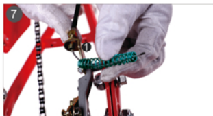
7. Put on the brake spring.
