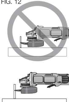
pressures encountered with surface grinding. Wheel breakage and injury may result.
