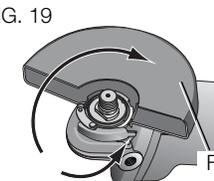
5. To remove the guard, open the guard latch, rotate the guard so that the arrows are aligned and pull up on the guard.
