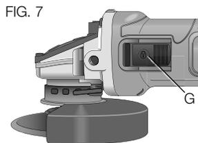
To start the tool, slide the ON/OFF slider switch (G) toward the front of the tool. To stop the tool, release the ON/OFF slider switch.
