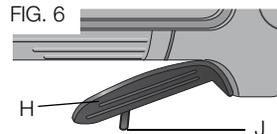
**⚠ WARNING:** Do not disable the lock-off lever. If the lock-off lever is disabled, the tool may start unexpectedly when it is laid down.
