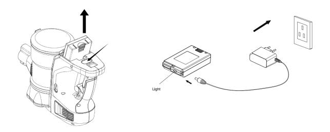
You can also charge the battery while it is inside the vacuum. The three blue indicator lights will indicate one by one to show the battery being charged. When the battery is fully charged, all three lights will stay blue.
