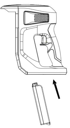
2. Install the dust container by inserting the clip into the main body, then put the upper side into place. It will "click" to secure.
