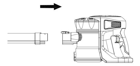
3. If using the motorized illuminated floor brush without the extension tube, simply attach it to the main body. It will "click" when secure.
