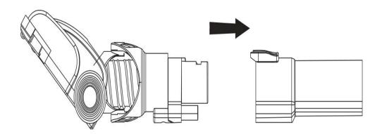
2. Attach the motorized illuminated floor brush and extension tube to the main body by slotting it into place.
