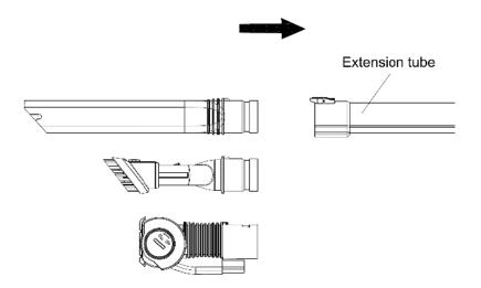
3. If using accessories without the extension tube, simply attach them to the main body. It will "click" when secure.
