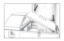
Place the small shield onto the main shield.
