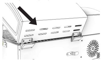
Over time the exhaust vents at the rear of the grill may get clogged. **IT IS VERY IMPORTANT** that these are cleaned properly and checked often.
