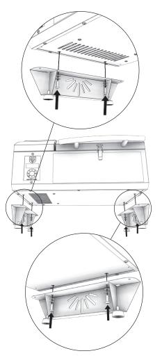
Note: Use the four rubber leg levelers to level the grill. Make sure the grill is always sitting level or is slightly tilted towards the drip pan.
