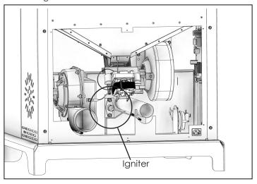
Disconnect the wiring leads connecting the igniter to the wiring harness.
