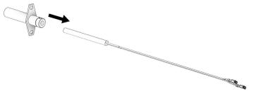
8. Slide the new igniter into the igniter housing. Leave approximately 1/4" between the end of the igniter and the igniter housing.
