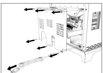
3. The igniter is located in the back center of the stove.
