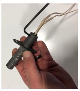
10. Replace the old gasket with the new gasket that is included with this kit. Slide the igniter housing into its original position in the back of the stove. Insert and tighten the two bolts that were previously removed.
