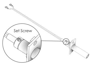
7. Remove the igniter from the igniter housing.
