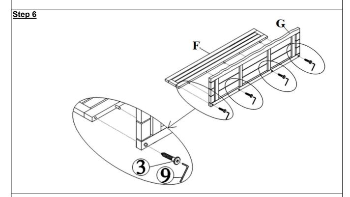
Assembly the Table Top ( G ) to the Back Panel ( F ) by using Allen Key (9) to tighten the Long Screws (3) in.
