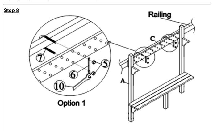
With assistance from your adult partner, stand pre-fixed table in Step 5, right side up. Attach the Table Support Bar (C) to your balcony (railing) by using Horseshoe Bolt (7), Plate (6), Nut (5) and Spanner (10) as shown in picture.
