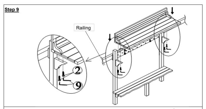
Assemble pre-fixed table from Step 7 and Step 8 together by using Long bolts (2) and Allen key (9) as shown in picture.
