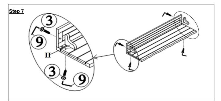
Assembly Upper Support Wings (H) to finish part in Step 6 by using Long Screws ( $\mathfrak{F}$ ) and Allen Key ( $\mathfrak{F}$ 9) as shown in picture .
