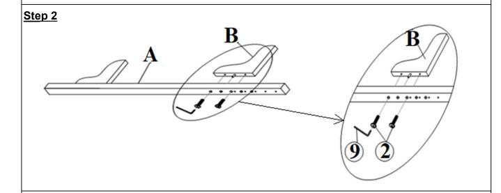
Customer need to check the railing height, matching to table height, before assembly of Lower Support Wing (B).
