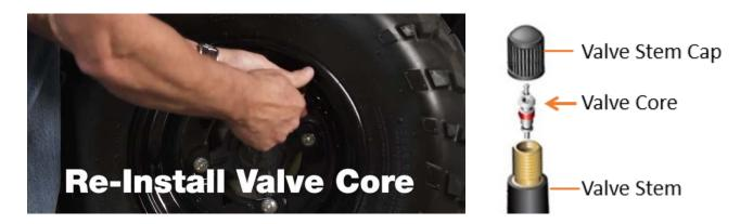
10. After filling the tire with the recommended amount of sealant, turn the bottle right-side up, and disconnect the bottle's tube from the valve stem. Insert the valve stem core into the open valve stem. Using the core removal tool, screw the valve stem core <u>clockwise</u> until tight.
