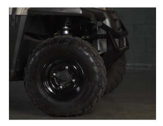
13. To fully distribute the sealant, rotate the tire several times (depending on the item, this multiple rotation can be done by driving, pushing, or by hand rotation).
