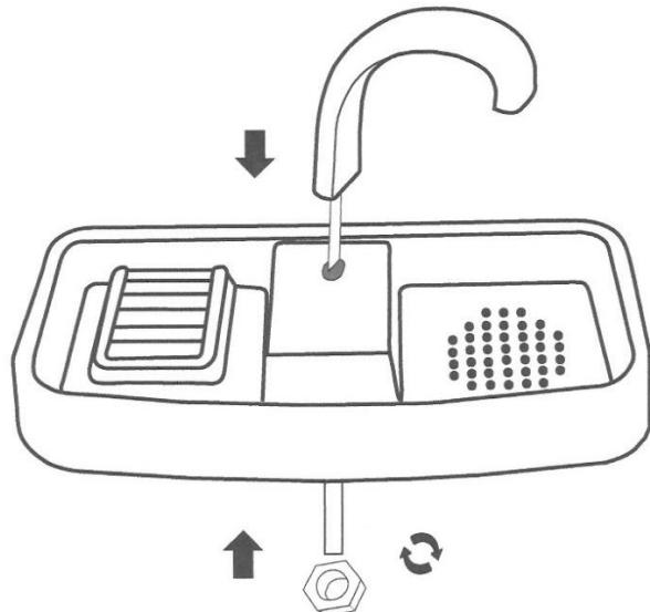
Insert the faucet tube into the hole on the top of the sink basin and complete the assembly by fastening the hex nut through the faucet tube and onto the underside of the basin.
