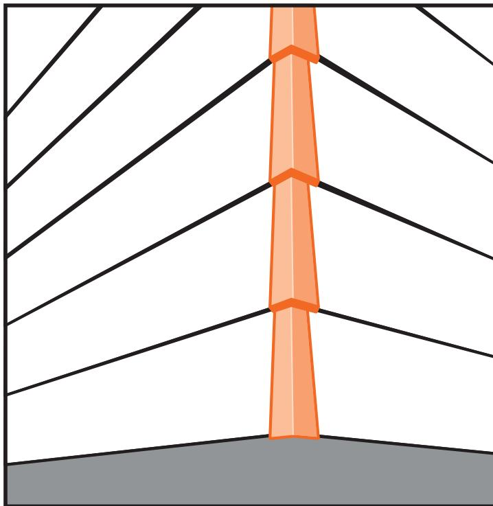
2. Continue working from the bottom up. While driving the nails pay attention to the vertical and horizontal alignment of the siding corner. Trim the last corner to fit.
