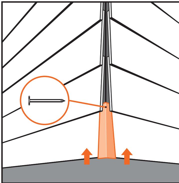
1. Start with the bottom course of siding. Carefully slide the first corner up and under the second course. Continue until the bottom wrap around lip is fully fitted to the bottom courses.
