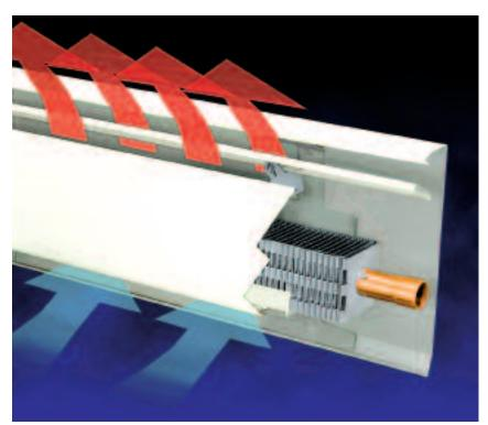
Wall streakage eliminated. Top panel and damper form a shield to keep dust from settling into baseboard interior, and to deflect heated air away from the wall, into the room. Back panel has no holes or slits to leak air behind the back of the baseboard causing wall streakage.
