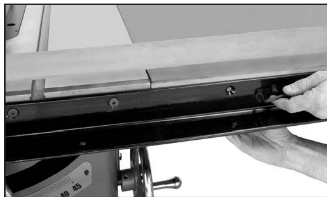
Figure 31. Aligning main extension table.
