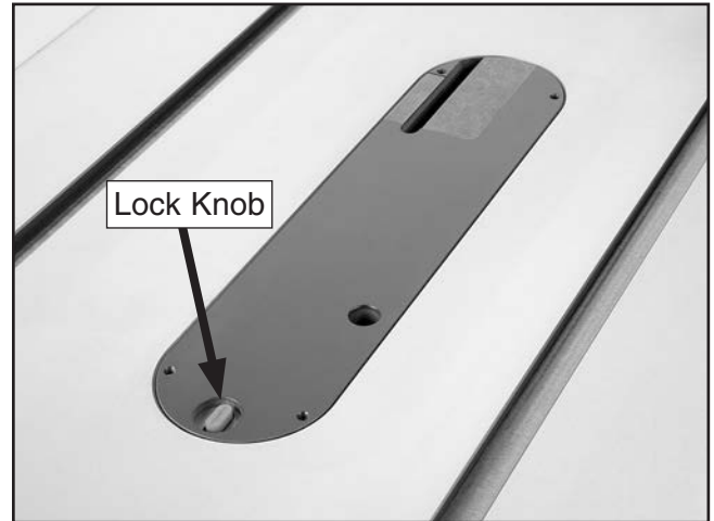
Figure 39. Insert lock knob unlocked.
