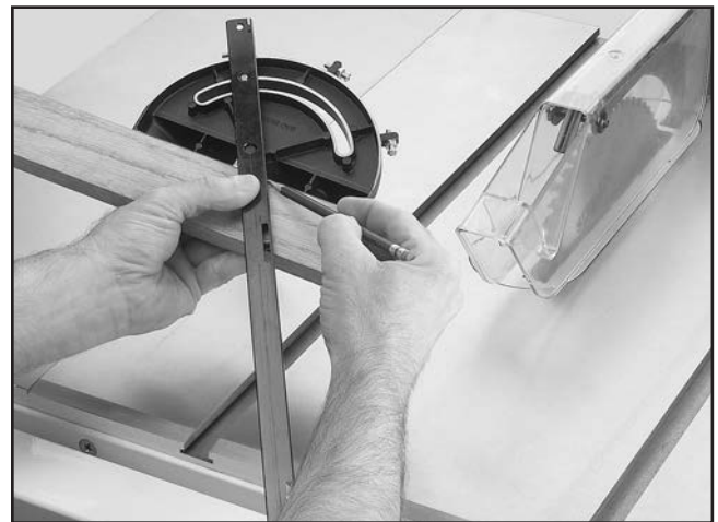
Figure 75. Example of marking miter line.
