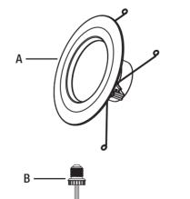
• The factory setting of the torsion spring clips is for a 6 in. housing.
