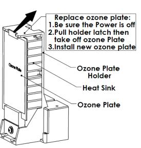
4. Install ceramic plate as in figure. Be careful not to drop the plate.
