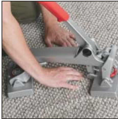
For pulling trimmed edges together
