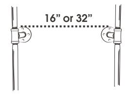
5. Place bracket assembly against the wall in the desired location, with the top hole of the flange set in the center of the stud. Mark the hole with a pencil. Now mark the bottom hole of the bottom flange. Place a level between the top mark and the bottom mark. Adjust position of the bottom mark so it is vertically level with the top hole mark.
