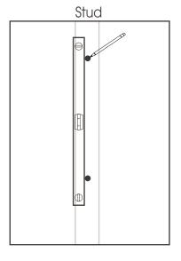
6. Using a level, mark the top hole for the other bracket assembly in the center of the stud where it will be installed. This mark needs to be level with the first top hole mark. Mark the bottom hole the same way; level with the first bottom hole mark.
