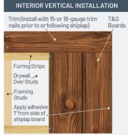
• The boards should be fastened in a similar fashion to interior wall studs. Adhesive may be used to reduce the need for fasteners.
