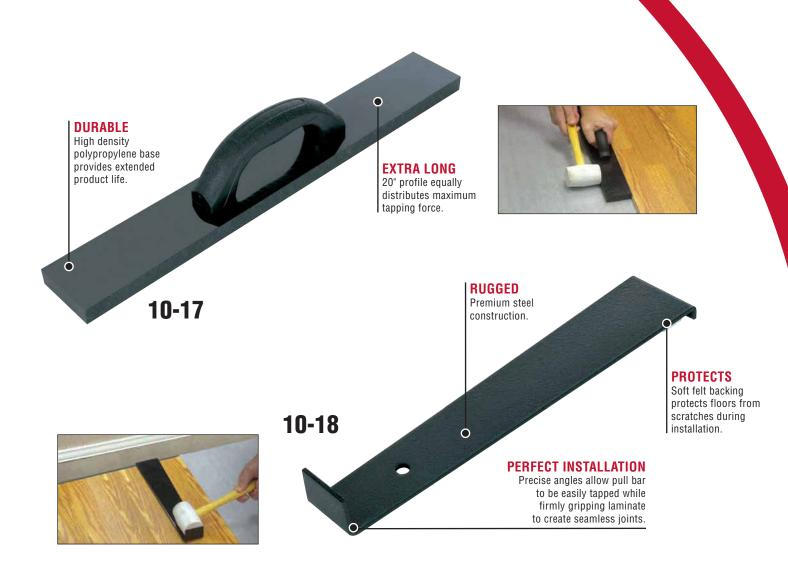
Used to install all brands of pre-glued tongue and groove flooring, these tools are essential for installing laminate flooring. The Tapping Block base is 20" long by 2.75" wide by .75" high for maximum impact distribution to eliminate damage to the groves of the flooring. The Pull Bar is a must for getting in between the wall and floor when the last plank is being tapped into place.
