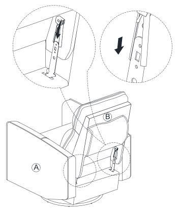
Attach the Back (B) to the Seat (A) by sliding the receivers into the mechanism posts located on the Seat (A).
