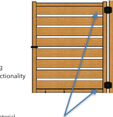
Hinges position should be installed as shown in drawing [3.5 inches from the top and bottom (B)]
