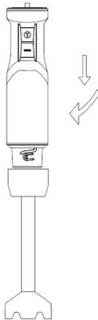
2. Insert the plug into socket. Press high-speed button or low-speed button to start the blender. When you press low-speed button, you can rotate the speed control knob to adjust the speed.
