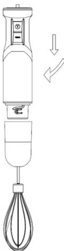
3. Press the switch to activate the handle blender, and press the high-speed button after 30 seconds to prevent ingredients from splashing.
