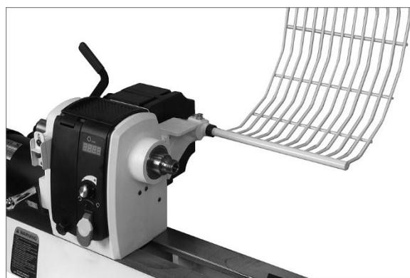
Figure 5-5: guard (optional) tilted back
