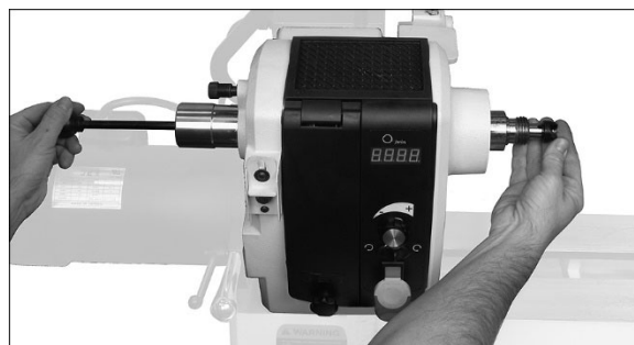
Figure 7-8: removing spur center
