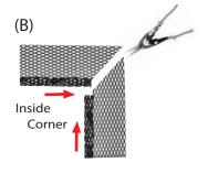
At the end of the gutter, cut the last gutter guard an extra 2 inches longer than the end of the gutter. Cut a notch on the back edge of the gutter guard (A) and on the front edge (B). Bend the end section down to create the end cap.
