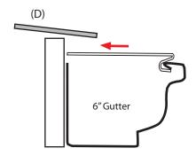
The Lock-In Gutter Guard comes with a pre-notched end that allows the guards to overlap, eliminating any gaps that would allow debris through the seams and into the gutter. As you install each section simply overlap the end with the previous section.
