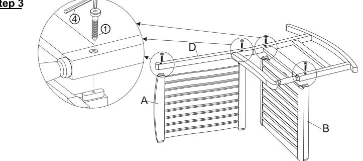
With assistance from your adult partners, put the tenon of Backrest Panel(A) and Seat Panel(B) into the mortise of Right Leg Panel(D) and attach using Screws (1) with Allen Key (4).
