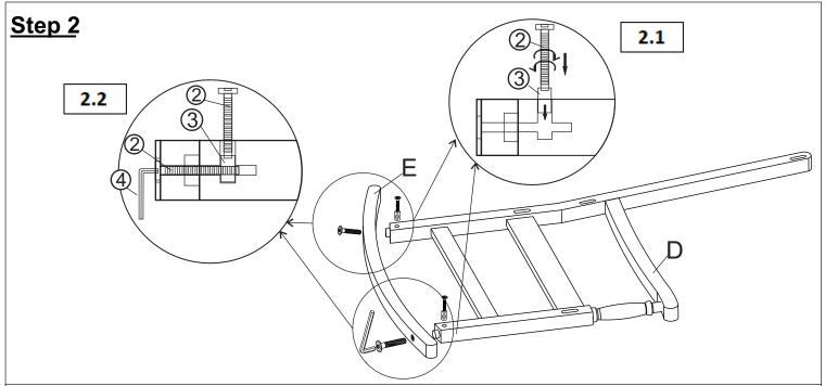
**2.1**) Insert Bolt (2) into Cross Dowel (3), then insert the Cross Dowel (3) into the housing on Right Leg Panel(D) as shown in above picture.
