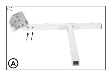
**Step 2.** Apply two 15/16" bolts (7) with a washer on each side of the Connection Block followed by the lock washer and then the nut for each bolt. Securely tighten both bolts with wrenches. Proper tightness will help keep the carrier quiet during use. See page 7 for details about attaching the Bogie Wheel (sold separately).
