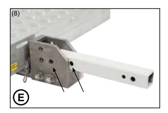
**Step 9.** The Hitch Bar should fit snugly so that your carrier is quiet. Install the last 15/16" bolt with a washer on each side, lock washer, and nut as previously done in Step 2. Tighten the bolt with a wrench and/or socket wrench.
