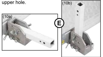
**Step 11.** Locate one Hanger Adapter (12) and install it on the carrier via the two holes near the spring handle. Tighten the Hanger Adapter with a screwdriver and wrench.
