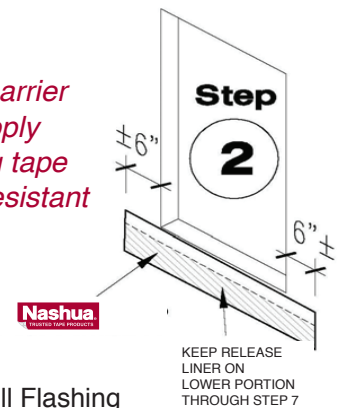
Figure 3 Apply Sill Flashing
