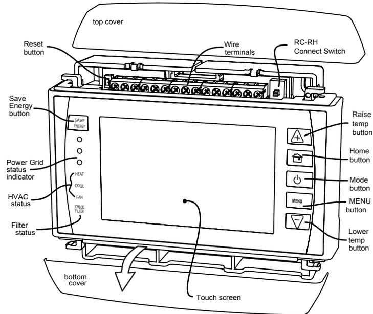
**Statement of use:** 100% Compatible with all popular residential HVAC systems; 24VAC single, two, three stage conventional heating systems (gas/oil/electric), heat pumps (single and two stage compression) and 1,2, or 3 stage auxiliary heat (electric or fossil), zoned forced air and zoned hot water (2 or 3 wire), millivolt systems (with 24VAC adapter), one or two stage cooling, and hybrid systems.
