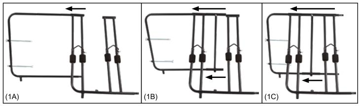
**Step 2.** Connect the bottom of the U-Frame to the bottom of the Main Rack Frame. Fit the Bottom Support Bar (G) into the brackets and secure with two Clip Pins (H).
