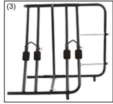
A. To connect the back U-Frame sections, fit one Spacer Bar (F) between the top bars and one Spacer Bar between the bottom bars. Secure with two Clip Pins (H) per bar.
