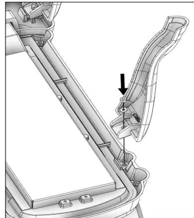
8. Carefully lift the stove upright and place in the desired location. Align the holes on the flue collar to the holes on the stove and attach using (2) two 1/4-20 X 1-3/4 screws.
