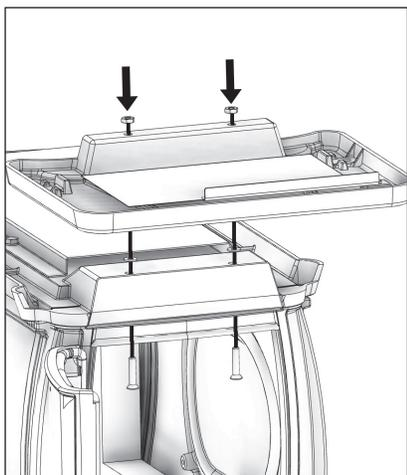
6. Attach the front legs to the hearth with two (2) 1/4-20 x 1-3/4 screws, two (2) washers, and two (2) 1/4-20 jam nuts. NOTE: Only one leg is equipped with a handle bracket. This bracketed leg is designed to be installed at the front right side of the unit.
