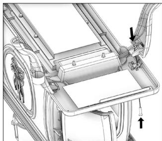
7. Attach the rear legs to the base of the stove with two (2) 1/4-20 x 1-3/4 screws, two (2) washers, and two (2) 1/4-20 jam nuts.
