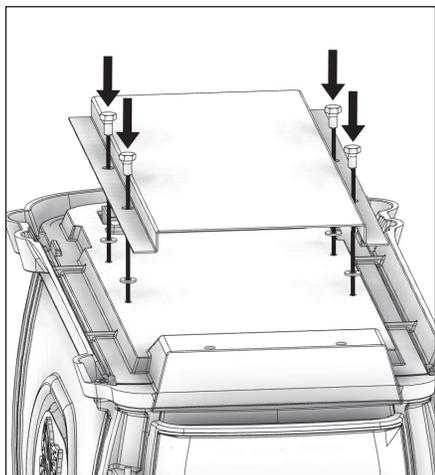
5. Attach the hearth to the bottom of stove using two (2) 1/4-20 x 1-3/16 screws, two (2) washers, and two (2) 1/4-20 jam nuts.
