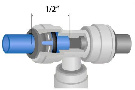
\*To connect, insert the tubing 1/2 inch deep until it's sealed by o-ring and locked by spider teeth.
