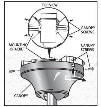
□ Lift the screw cover ring up over the screws and twist counterclockwise to secure in place.
