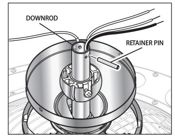
**STOP** For Canadainstallations,refer to the Canada Installation Addendum and install the support cable on theretainer pin now.
