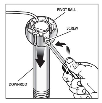
$\hfill\square$  Remove the retainer pin from the downrod.
