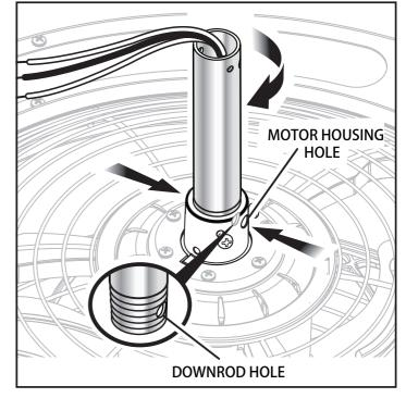
□ Install the clevis pin through the holes in the motor housing and the downrod, then reinsert hitch pin. Retighten the lock screws to secure.
