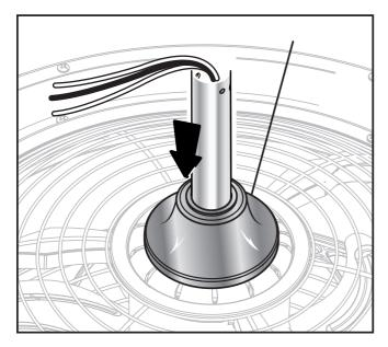
□ Carefully feed the fan's electrical wiring through the center arm support, then install the support with the cupped side facing up.
