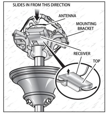
Slide the canopy up into place and rotate clockwise to lock to mounting bracket assembly. Reinstall the two s crews (M4 x 6 mm) removed previously and tighten securely.
