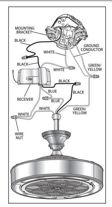
Spread the wires apart so the green/yellow and white wires go to one side and the black and blue go to the other, then carefully tuck all the wire connections up into the outlet box. **NOTE:** Orient the wires so the wire nuts are facing up and are not touching each other. This will help minimize potential noise once the installation is complete.
