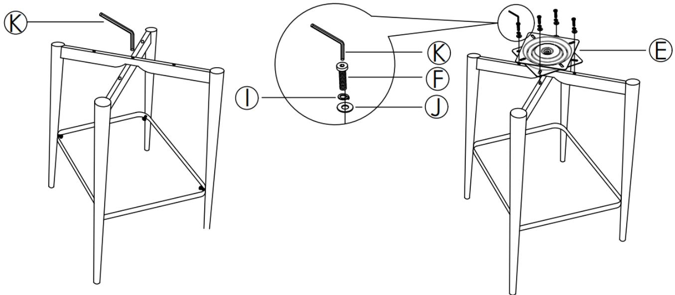
④ Put assembled legs in step 3 on a flat surface. Push legs up or down as necessary to level. Once level, tighten all bolts.
