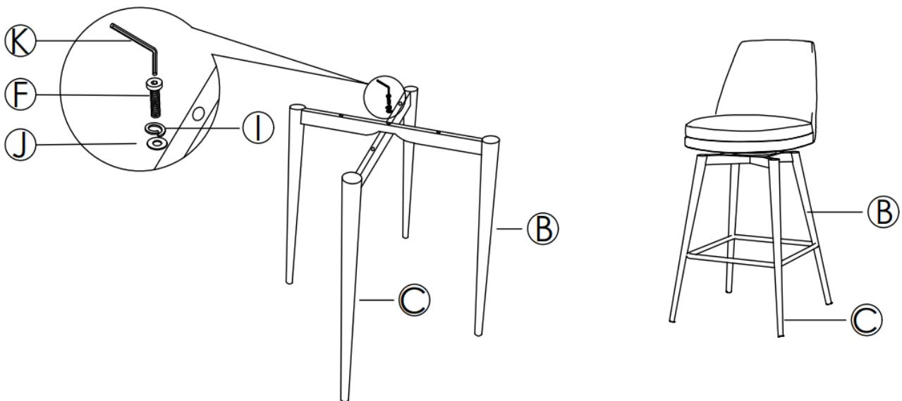
② **Loosely** attach the bolts (H) one by one and **keep them loose**. **Do not fully tighten**. After **loosely** attach the first bolt, move on to the diagonal bolt. After all 4 bolts are attached, use allen wrench (K) to tighten.
